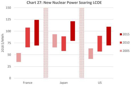
Note: cost ranges for discount rates of 5% (minimum) and 10% (maximum) Source: IEA/NEA, <u>Projected Costs of Generating Electricity 2015</u> (September 2015)
