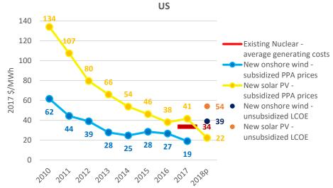
Chart 25: New Onshore Wind and Solar PV Putting Heavy Stress on Existing Nuclear Power in the
