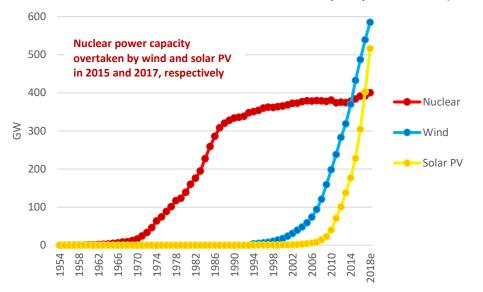
Chart 3: World Nuclear, Wind, and Solar PV Cumulative Capacity 1954-2018e (Dec. 3)
